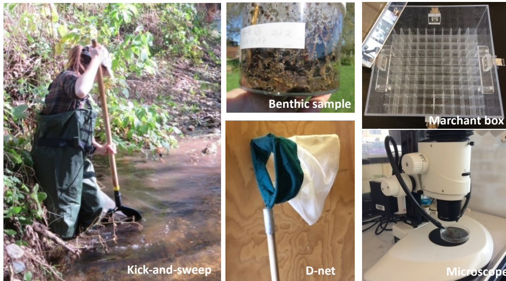
Figure 20 – Techniques and equipment used when sampling BMI using the CABIN protocol. From left to right: collecting BMI using a kick-and-sweep technique; collected BMI sample; D-net; Marchant box; microscope.
